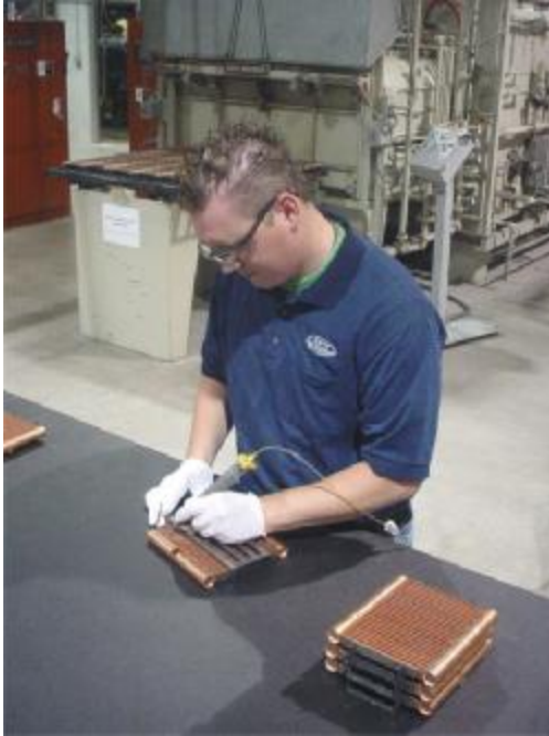
Vintage Air makes a climate control system that is popular with OEMs as well as the aftermarket. Brazed copper-brass technology allows for a compact and durable heat-exchanger core.
