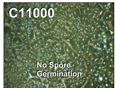
Figure 2. Aspergillus niger spore germination on aluminum and copper. A fungal broth of 10^6 spores were placed onto aluminum and C11000 copper, incubated at 37°C (image taken at 100X) after 10 days. No spore germination was observed on the copper, while hyphae formation was clearly visible on the aluminum.
