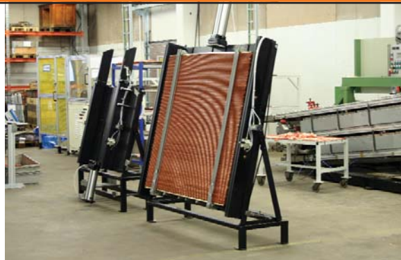
Fins, tubes and side plates are assembled together on a core assembly table. This large radiator core is ready for brazing.
