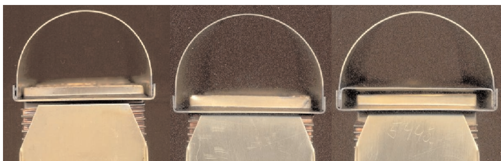
Stress at the tube-header joints can be reduced using new header designs. Stresses due to (a) narrow header width can be reduced with (b) extra header width and (c) an extra header.
