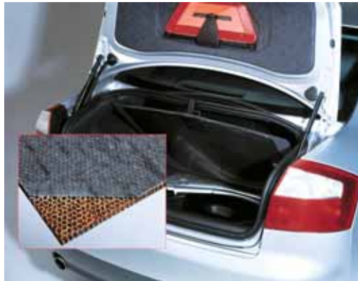
An Audi A4 spare tire cover uses Bayer's Baypreg F sandwich composite, which includes glass mats and paper honeycomb.
