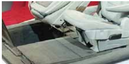
Bayer's HD-SRIM and glass mat reinforcement for the load floor of this DaimlerChrysler minivan provides a weight savings versus a steel panel.
