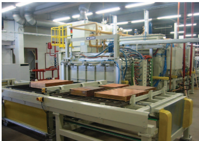
Charge-air coolers ready to be fed into the Seco/Warwick three-chamber brazing furnace. The midsize volume-production furnace is semi-continuous, allowing easy loading and unloading from both front and rear, which can significantly reduce process times and increase capacity.
